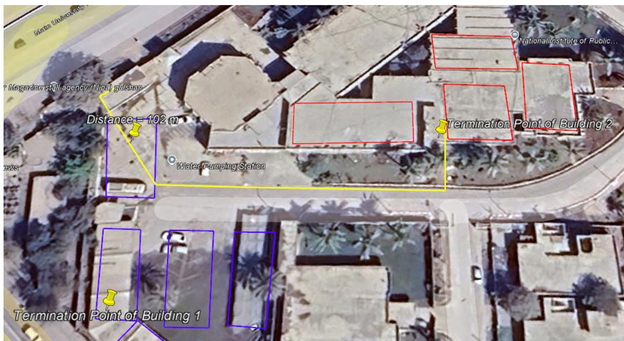
Figure 4: Termination Point of Both Buildings and Additional Cable Details
